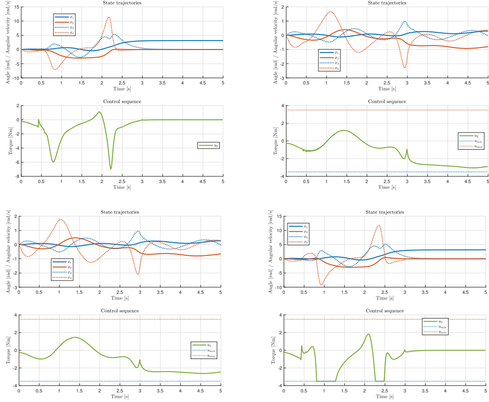
Figure 4.4: Trajectories of the acrobot under: no constraints (top left), naive clamping (top right), squashing function (bottom left), constrained quadratic programming (bottom right).
